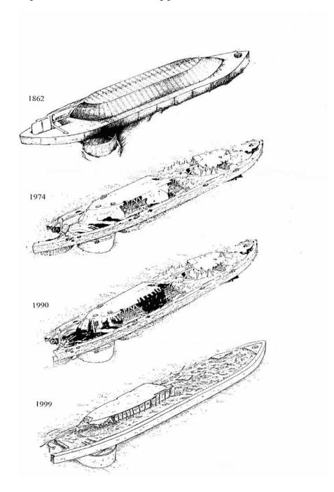
**LEFT:** *Monitor*'s hull began to deteriorate at an accelerating rate during the 1980s and 1990s. Line drawing depicting the rate of deterioration (*Monitor* Collection, NOAA).
