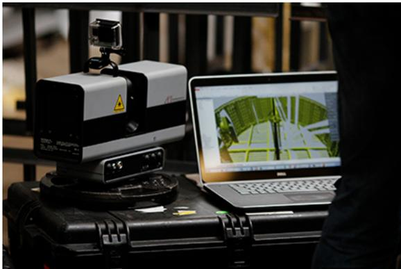
3-D model on computer screen details the inside of the turret. Photo: API Services
