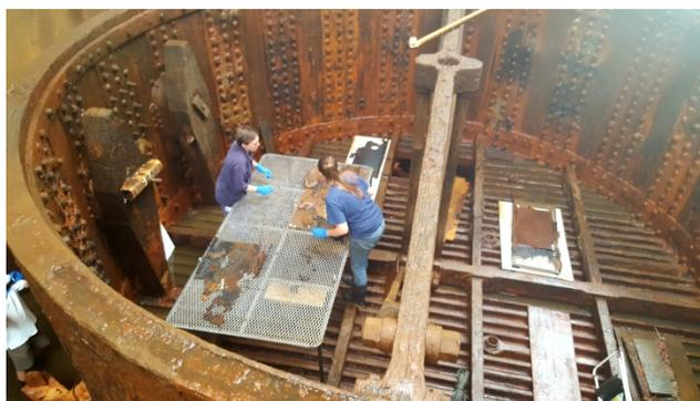
Conservators place the remnants of two nut guards removed from inside of the turret and place them on a metal screen for further conservation. Photo: Ricles, NOAA
