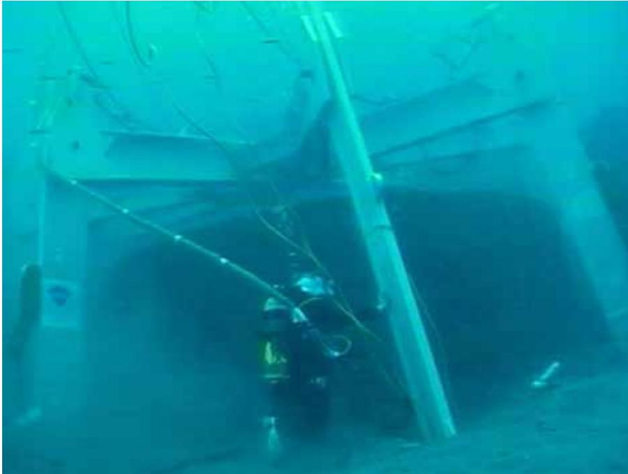
LEFT: A U.S. Navy diver works to secure the spider to the *Monitor's* turret in preparation for lift (NOAA).
