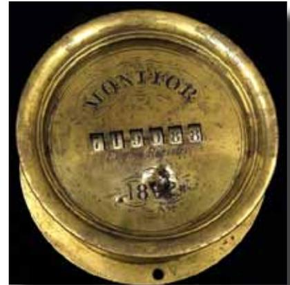
**ABOVE:** The conserved engine register was removed from the *Monitor's* steam engine. It was the first piece of the ship recovered with the vessel's name on it (The Mariners' Museum).
