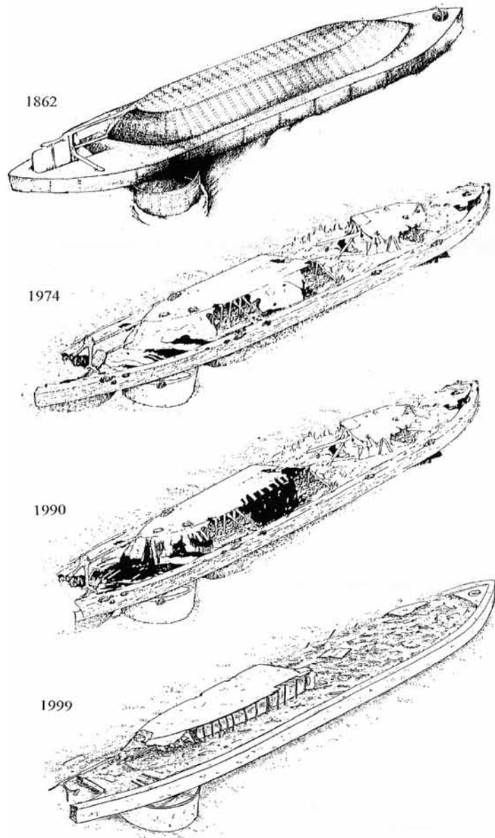
**LEFT:** *Monitor's* hull began to deteriorate at an accelerating rate during the 1980s and 1990s. Line drawing depicting the rate of deterioration (*Monitor* Collection, NOAA).
