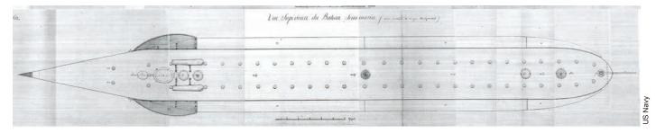
Figure 40. Schematics of USS Alligator: The U.S. Navy's first submarine as designed by Brutus de Villeroi, 1863.
