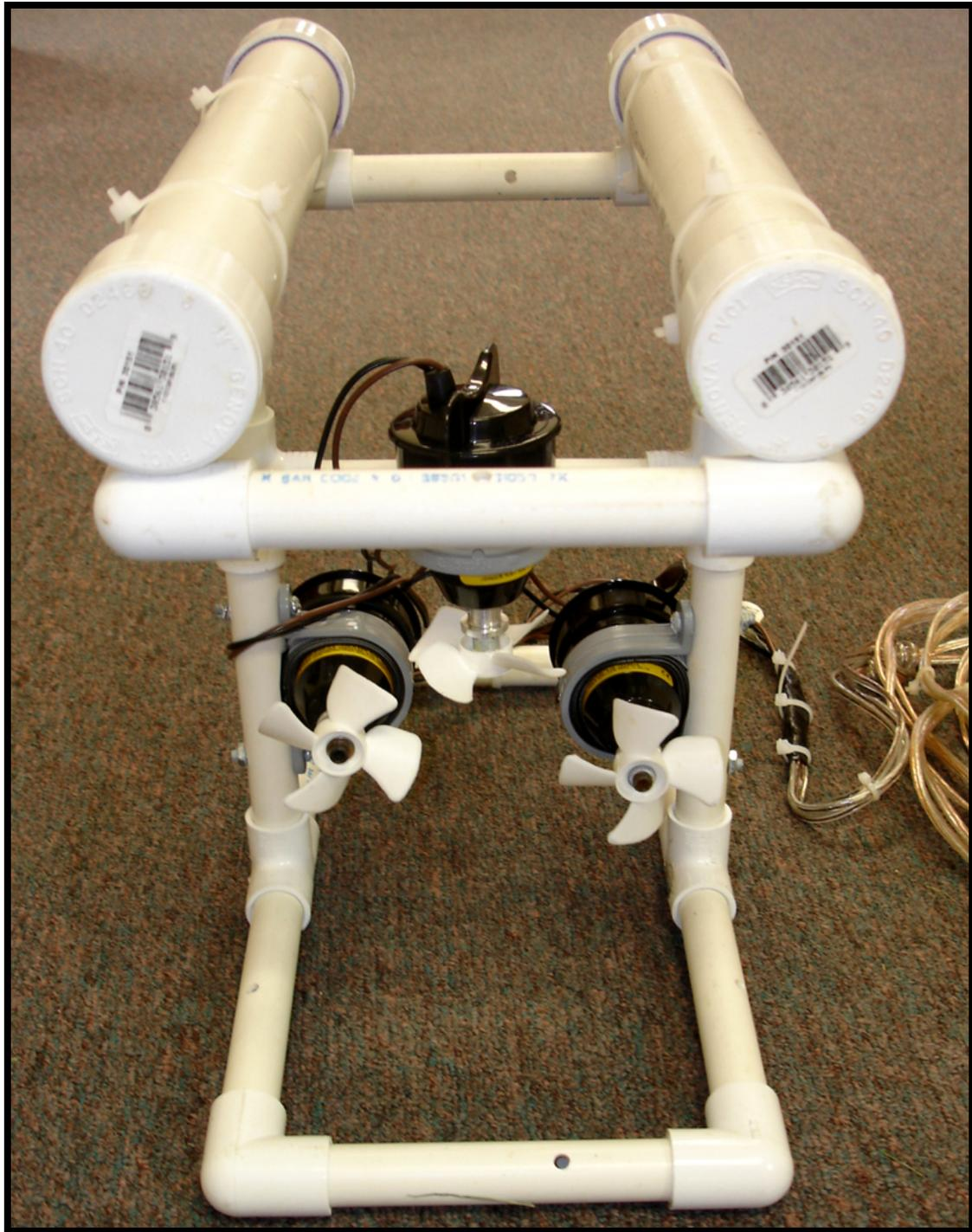
**Figure 1.3: In this front view of the ROV you can see that three thruster assemblies have been constructed and attached to the area inside of the frame. The function of the frame is to provide structure for the ROV and protection to the propellers which allow it to move through the water.**
