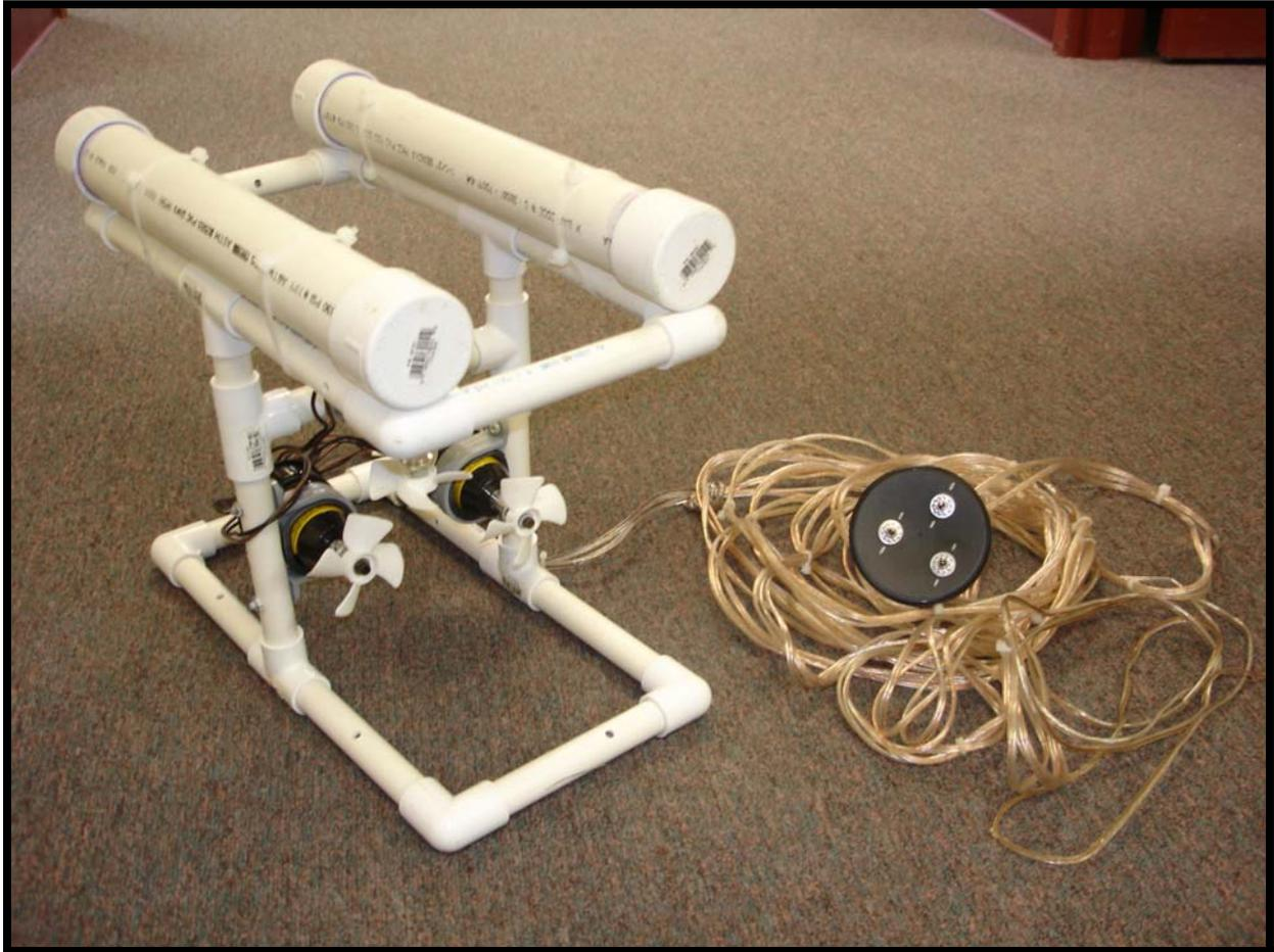
**Figure 1.2: This is a side view of an ROV created from parts described in the following pages. The buoyancy pontoons are attached to the PVC frame with plastic tie wraps. A bundle of three pairs of speaker wire transfer the information from the controller jar to the underwater robot.**
