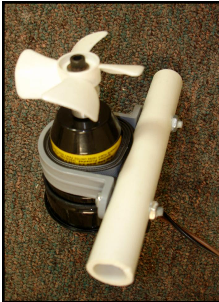
**Figure 1.16** The rubber tape seen here allows the cartridge to be tightened against the PVC frame.
