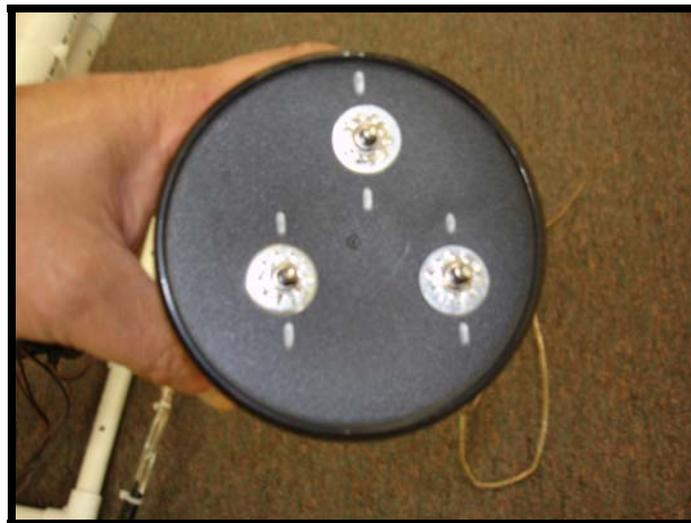
**Figure 1.6: The labeled controller jar lid. The silver vertical lines show the direction that the switches can be pushed or pulled.**
