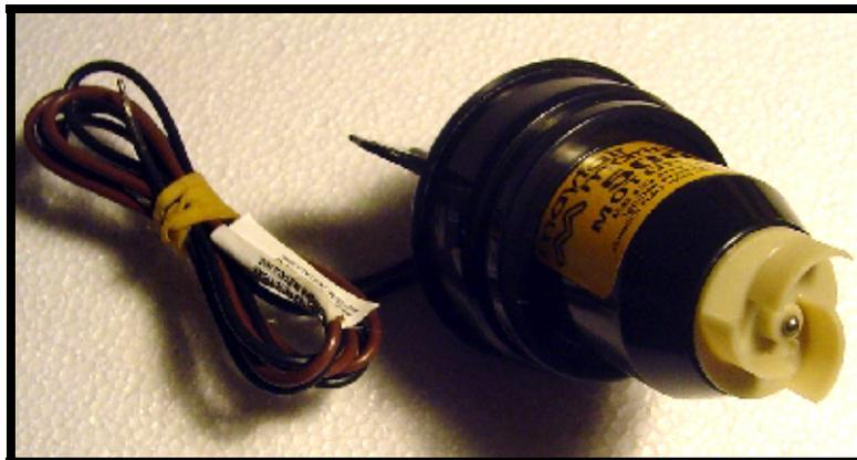
**Figure 1.13** The Bilge Pump Cartridge used for the thruster motors.
