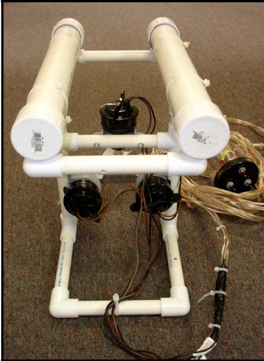
**Figure 1.4: This is a rear view of the ROV. The wire tether is attached to the thrusters from the rear. This enables the ROV to move forward without getting tangled. The tether will have to be managed manually (i.e. by hand) when the thrusters are operated in reverse.**
