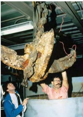
The *Monitor's* anchor was a short, flour-fluked anchor weighing over 1,000 pounds. It was unique in its design. The anchor was recovered in 1983, just south of the bow of the wreck. It was still attached to the ship and the anchor chain had to be cut in order to raise the anchor.
