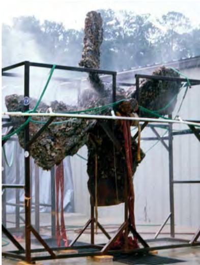
The *Monitor's* propeller was designed by John Ericsson as a four-blade, 4,600-pound, cast-iron screw propeller that was nine feet in diameter. Ericsson's revolutionary design was more efficient than a paddlewheel and allowed the engine to be mounted below the waterline so that it was protected from enemy fire.
